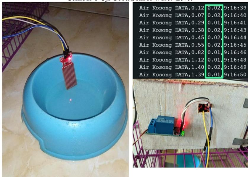
Gambar 9 Uji Coba Sensor *Water Level*
